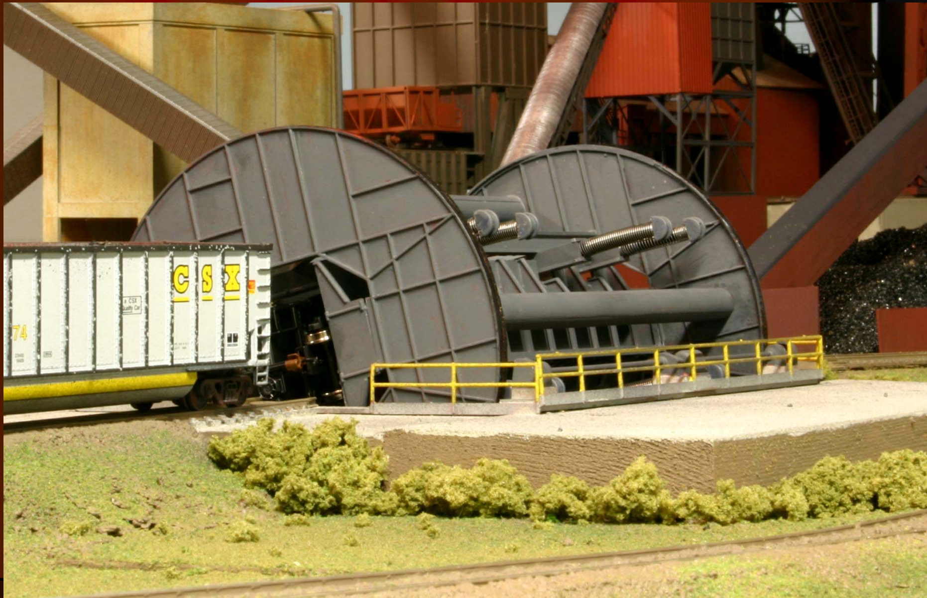
Rotary dumper in action
