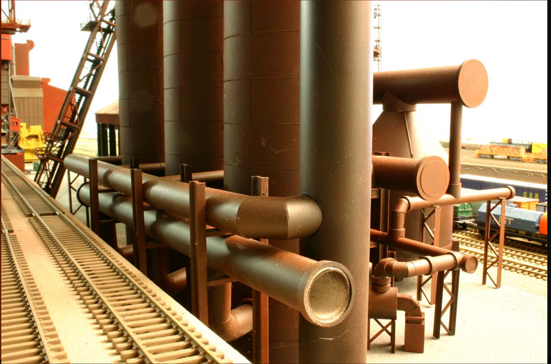
Close-up of heating exhaust (top pipe, into stack) and cold blast main (bottom pipe), with highline in foreground
