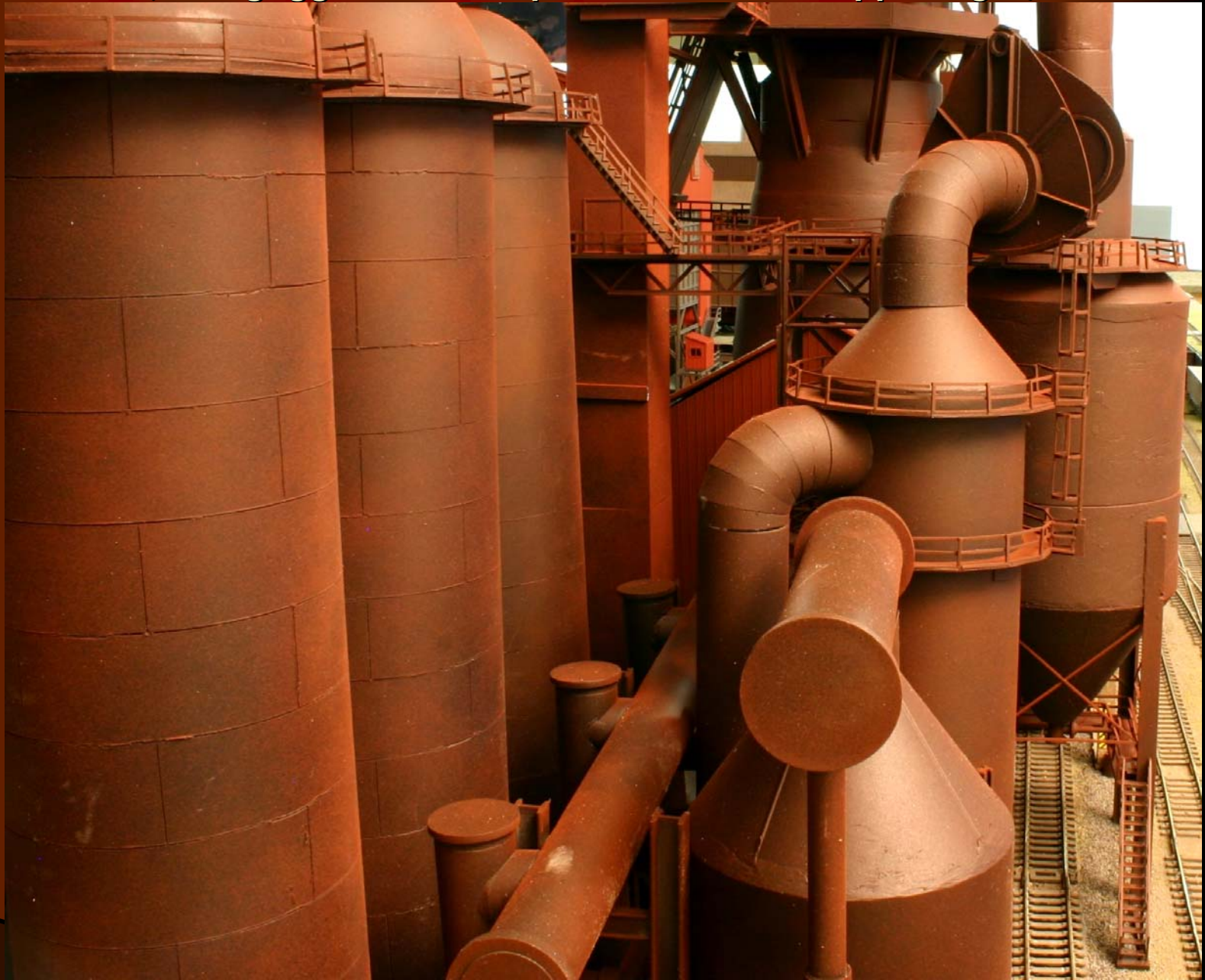
Close-up of stoves and hot blast main (note goggle valve atop dust catcher in upper right)
