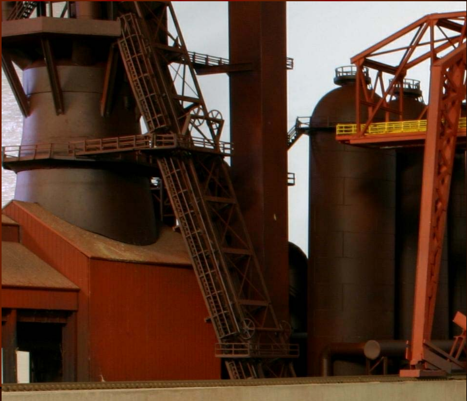
Close-up of skip hoist and safety-caged stairway
