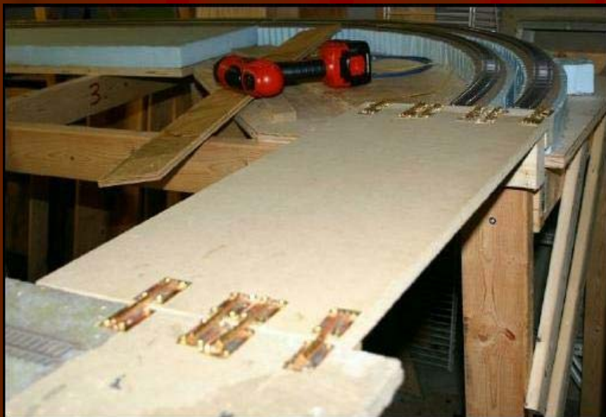
Views of lift-out platform, before and after installation of track and wiring
