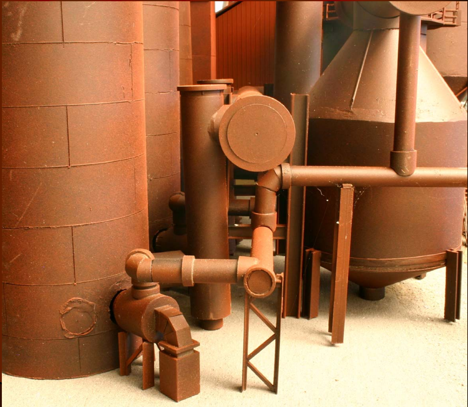
End view of hot blast main, with return gas piping and burner
